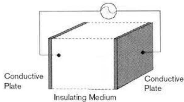
77. Principal uses for capacitors include storing electrical charges, conducting alternating current (AC current), and blocking or separating different voltage levels of direct current (DC current) sources. Capacitors are differentiated based on their construction, with different materials providing unique characteristics;
