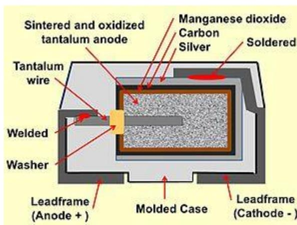
93. Tantalum capacitors are, however, susceptible to short-circuiting or catastrophic thermal runaway failure and destruction by fire if subject to inconsistent voltage or voltage spikes, as such inconsistencies can tax and break down the capacitor's extremely thin dielectric;
