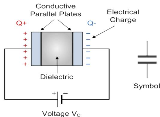
79. Generally, a capacitor is used in an electric circuit to store electrical charge. In this regard, it is distinguished from a battery in that a battery provides electrical charge to an electrical circuit;
